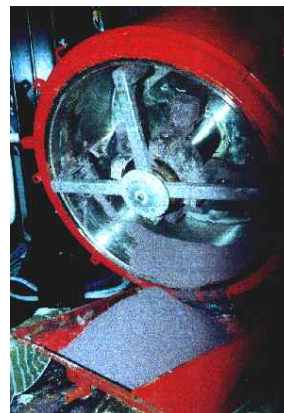
Scraping blades, adjustable and removable Shaft gaskets fluxed by compressed air Start and stop : manual or automatic Motor power: 370 W
